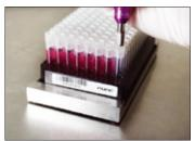
Caps are replaced using the single or multiple head screwdrivers. Vials are locked into the rack, which ensures that they do not fall out during transport in the lab or storage. The snap in the rack also retains the vial in the rack when the cap is mounted and the screwdriver is removed.
