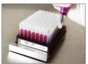
Removal of caps can be easily automated using a socket that snaps into the cap. Our partners offer 96 head decappers using this technique.
