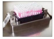
The Nunc tube selection tool has a cut-off corner that ensures that the rack and tube selection tool orientation is always aligned when the levers are pressed out of the rack and lifted up for easy retrieval. The rest of the rack is rapidly returned to the freezer to avoid significant thawing.
