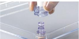
CLICK a CPC connector on your media bag into a male CPC port. A semi-closed system for GMP production.
