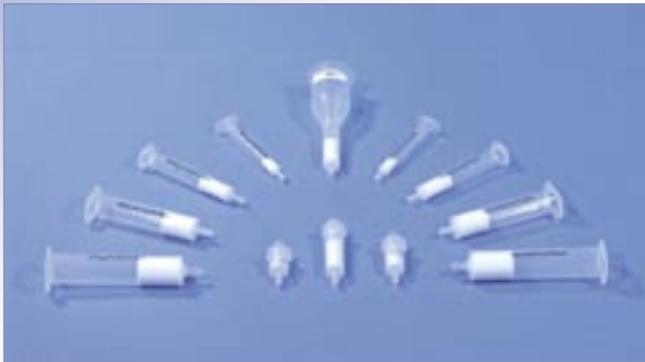
Solid phase extraction (SPE) is a powerful method for sample preparation and is used by most chromatographers today.
