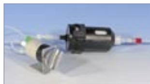
VALCO Cheminert® injection valve with sample loop
