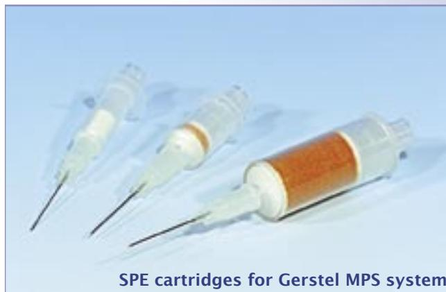
SPE cartridges for Gerstel MPS system
