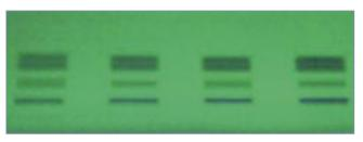
Identification of separated substances is possible via the  $R_{\rm f}$  value compared to the pure compound, which is often applied simultaneously on the same plate.
