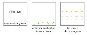
Another method for sample concentration is a short pre-elution (few mm) with a solvent, in which all substances have a high  $R_{\rm f}$  value.
