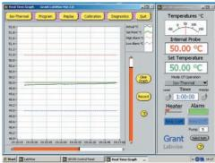
Real time temperature monitoring showing high/low alarms and 'zoom-in' facility
