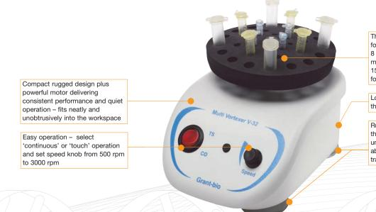
The 32-socket universal platform for three tubes sizes (16 x 1.5 ml, 8 x 0.5 ml, 8 x 0.2 ml) and a tip for mixing individual tubes up to 15 ml provide maximum flexibility for different applications
