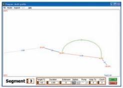
Multi-segment program with cycled segment (simple 'drag and drop' operation to change all parameters)
