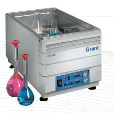
**Combined orbital/linear shaking bath OLS200** for optimisation and flexibility of application
