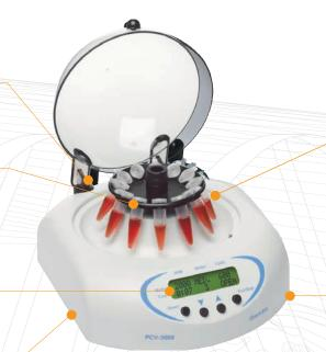
after mixing allows lower reagent volumes to be used. Because of its powerful G force and accurate control of spin and mix parameters, the Multi-spin<sup>TM</sup> can be used with volumes as low as 5  $\mu$ L.
