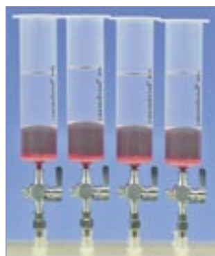
CHROMABOND® PTL in action: organic upper phase (colourless), aqueous lower phase (red)
