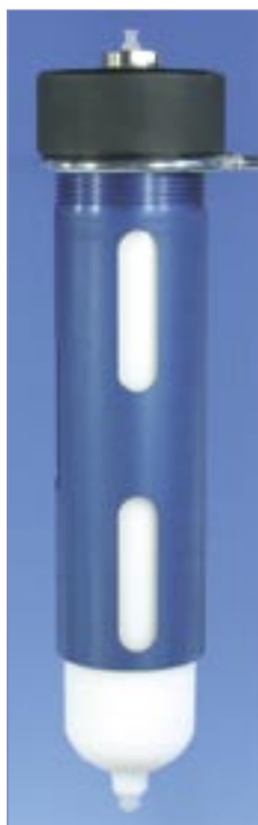
Flash holder 750 with cartridge (65 mm ID)
