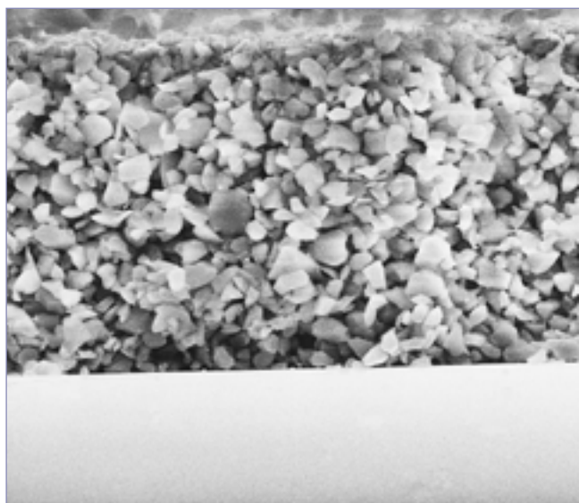
Electron microscope photograph of a cross section through a glass plate with silica layer (magnification x 500)
