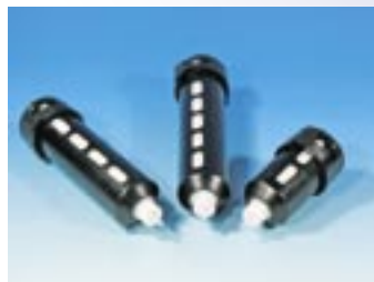
CHROMABOND® Flash C-90, C-180, C-240 cartridges with the corresponding Flash holders
